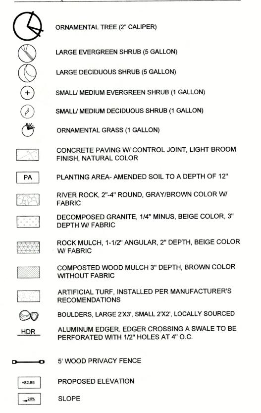
NOTE: ALL PLANTING AREAS TO BE IRRIGATED BY AN AUTOMATIC SYSTEM WITH CONTROLLER. PLANTING TO RECEIVE DRIP IRRIGATION.
